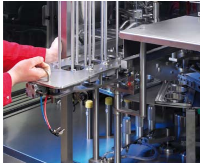
Cup setter with sliding frame
