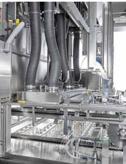
double pulsed light high-performance UV(C) cup sterilisation with guaranteed sterilisation rate LOG 4
