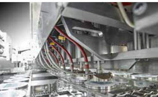
leak test station
