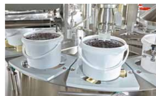
Dosing station with maximum dosing accuracy
