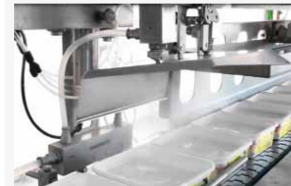
Spraying station for anti-stick
