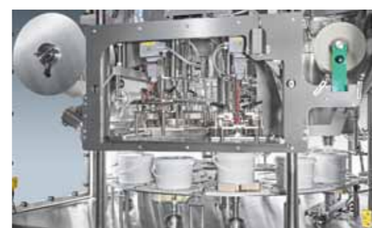
Double cutting /sealing station for closing buckets with peelable film from the reel.
