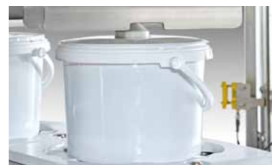
Leak test control of the sealing
