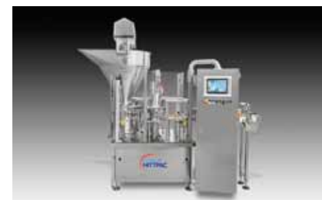
GRUNWALD rotary-type machine for filling pâté in sterilisable aluminium and plastic cups
