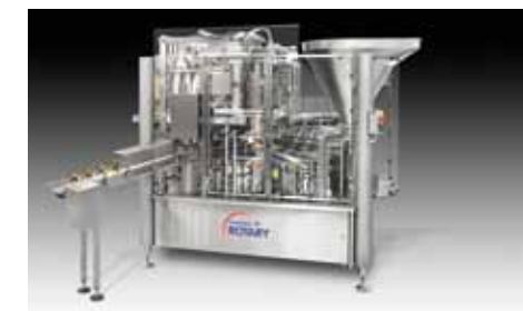
Exhibition machine at IFFA 2019: 4-lane cup filling and closing machine GRUNWALD-ROTARY 6.000 Product: Delicatessen salads Packing: 2 different round cups, seal lid and snap-on lid closure Filling volumes: 30 - 120 grs
