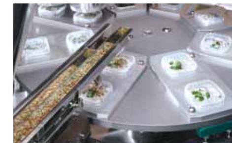
View into a GRUNWALD rotary-type machine with garnishing station for pepper cubes (on the right of the photo) and spice mixtures (on the left)
