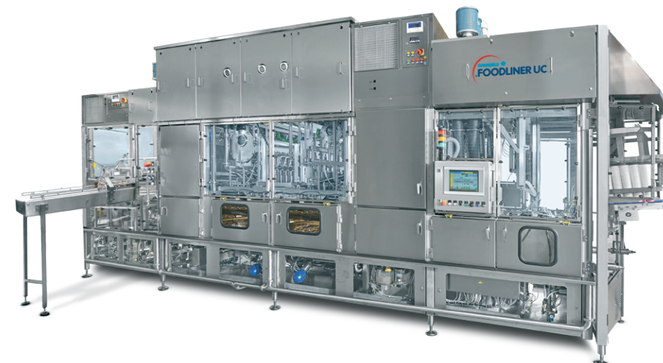
Photo on the left: The next ultraclean (UC) machine generation: fully-automatic cup filling and closing machine GRUNWALD-FOODLINER 20.000 UC in 10-lane design with integrated tray packer for dairy products
