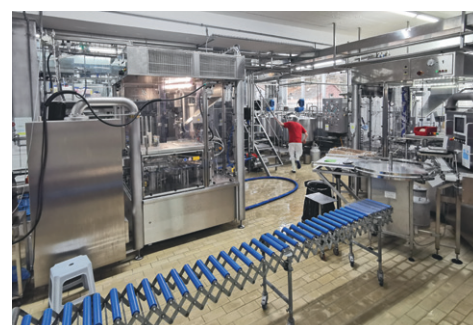
Photo at the top: View into the "foxhole" as Fuchs Dairy like to call themselves and on the two rotary-type cup fillers type GRUNWALD-HITTPAC AKH-059
