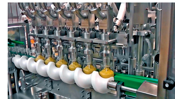
Photos above: GRUNWALD-SERVODOS 6-head filler with different bottle formats during the filling process
