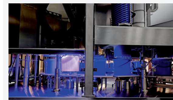
UVC sterilisation on rotary-type bucket filler GRUNWALD-ROTARY XXL
