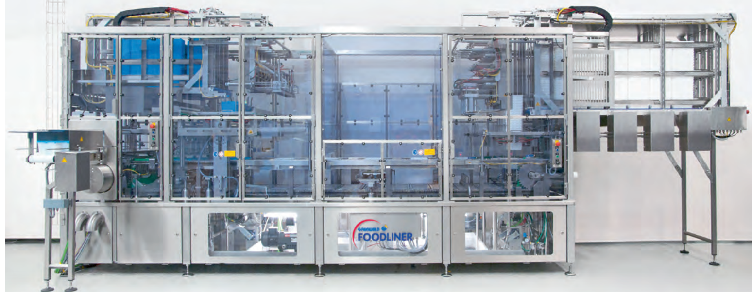
4-lane high-speed linear machine GRUNWALD-FOODLINER 6.000 with 3rd party filling system for soap capsules
