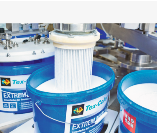
Filling station guaranteeing maximum dosing accuracy ( \leq 0.1\% standard deviation)
